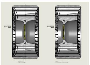
The offset of a wheel is the distance from the hub mounting surface to the center line of the wheel. The wheel offset, typically measured in millimeters, results in a positive, negative, or zero offset.
