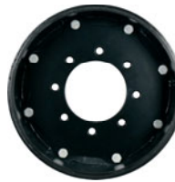
Hub Adapter MSPN 47868 CAI 291074 12 mm thick 1015 carbon steel / reversible 6.0" (152.4 mm) center dia. 8 x 8.0" bolt pattern 0.67" (17 mm) bolt holes, tapered Use adapter to change offset on 8 x 8.0" standard fitment size
