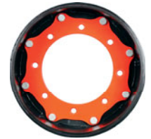
Hub Adapter MSPN 47462 CAI 481115 12 mm thick 1015 carbon steel / reversible 9.0" (228.6 mm) center dia. 8 x 10.75" bolt pattern 0.67" (17 mm) bolt holes, tapered Fits some Bobcat machines
