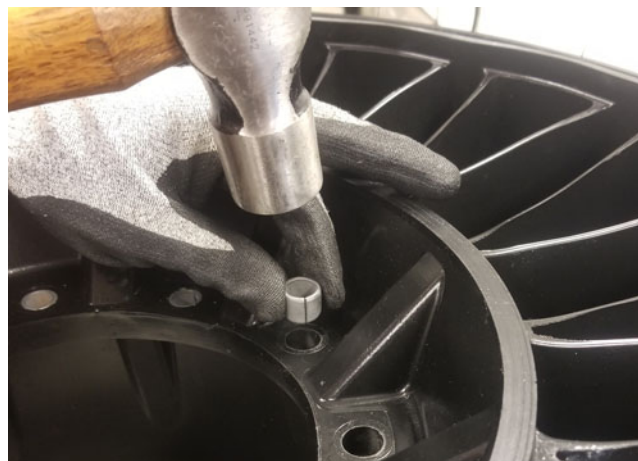
Above: Tapping in a compression limiter using a small hammer.
